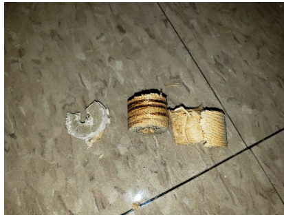
Floor Core non-Asbestos
